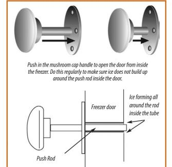
As warm air enters the tube from outside the freezer, water drips around the push rod and freezes. Ice builds up as more water drips and freezes. The rod cannot move with the block of ice around it.
