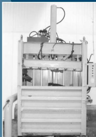
previous occasions, the ram became wedged sideways when compressing uneven loads, and a metal rod was used to pry it back into place. The bale compactor was not certified nor designed by an engineer, and had been in service for only seven months at the time of the accident.
