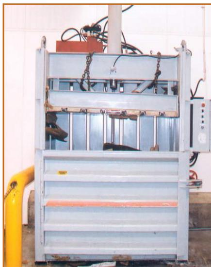
The unit worked in such a way that when cardboard was piled evenly in the chamber, the plate could come down and crush the cardboard without putting stress on the cylinder rod and connection pin. If, however, cardboard was not placed squarely in the middle of the chamber when the plate was lowered, it compressed the cardboard unevenly, causing stress at the joints.
