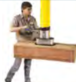
Vacuum Lifter Handles sacks and bags that are hard to grip by hand. They can also be very useful for handling large and heavy items.
