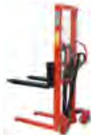
Manual Pallet Stacker Raises and lowers materials to the appropriate height.
